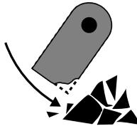
The surface of the material will become deformed or locally fractured and even break away when exposed to impact and/or high pressure conditions.
