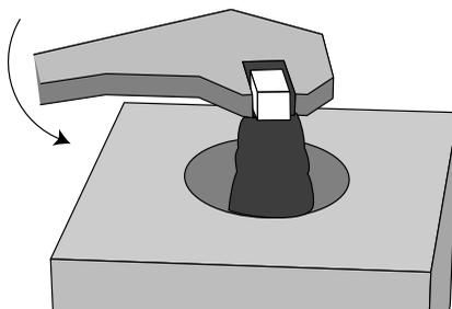
Extraction of broken bolt using OK 68.82.
