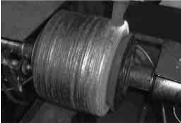
Hard-facing spin-wheels that are used in the manufacturing of mineral-wool. These wheels can be preventively maintained by adding several layers of Filarc 6166S or OK Tubrodur 15.85 or OK Tubrodur 15.91S.
