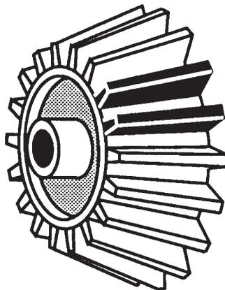
Repair of broken teeth in gear with OK 68.82.
