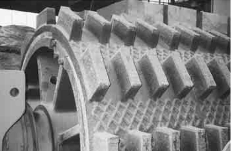
Crusher. Teeth: OK 86.20 buffer layer, OK 84.78 hardsurfacing.
