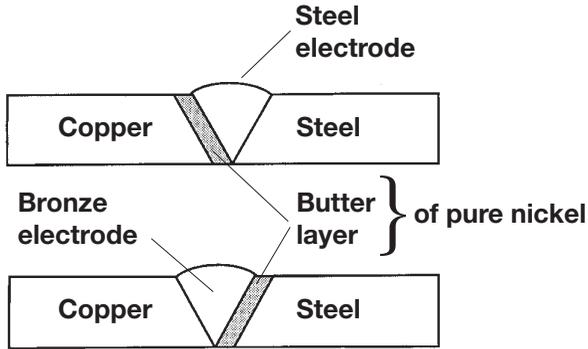
When buttering copper or bronze, preheating to 300–500°C should be applied. Thin material may be heated only around the starting area.
