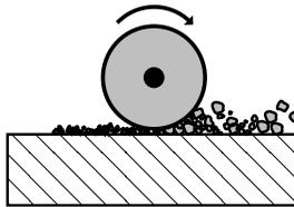
This type of wear occurs when small, hard, abrasive particles are forced between two metal parts and crushed in a grinding mode.
