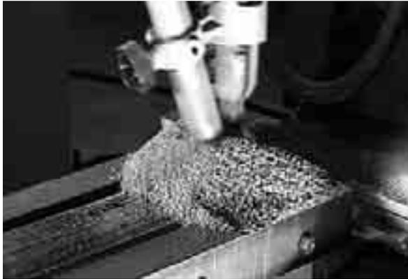
Hard-facing method that uses unalloyed wires together with alloying fluxes to obtain different hardness levels.
