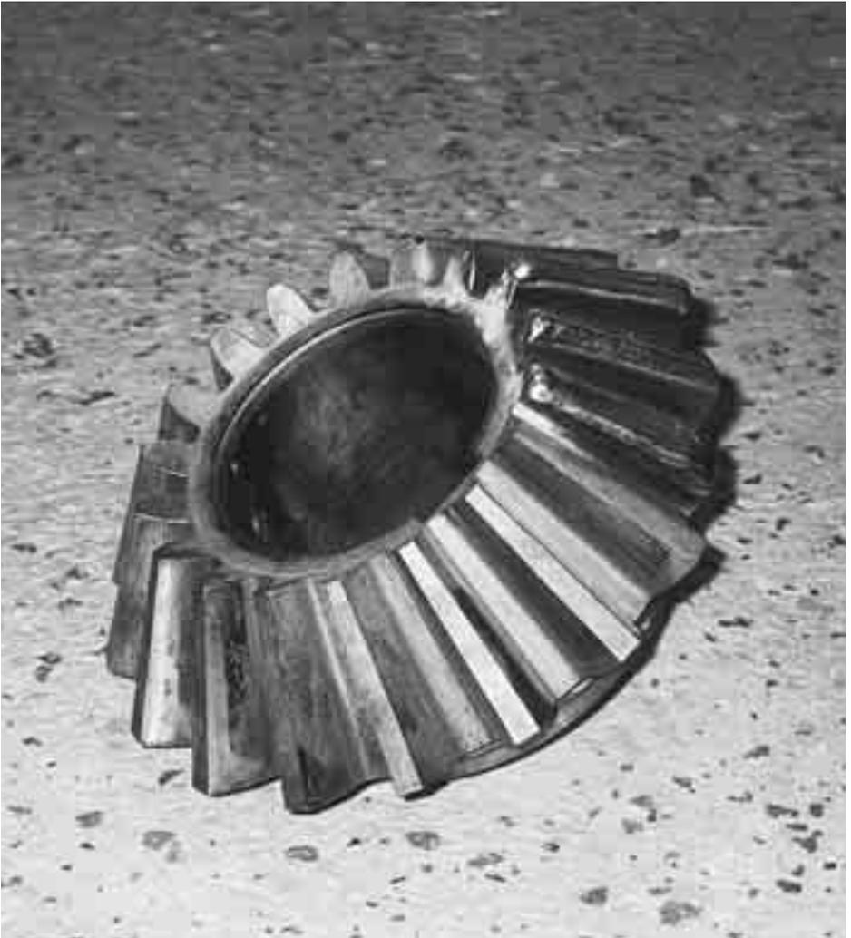
Gear drive. Rebuilding using OK 68.82.
