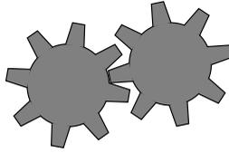
Wear from metal parts that roll or slide against one another, such as shafts against bearing surfaces, chain links against a roll, sprockets, steel mill rolls.
