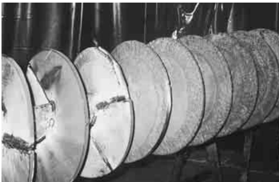
Feeder screw: OK Tubrodur 14.70 hard-facing.
