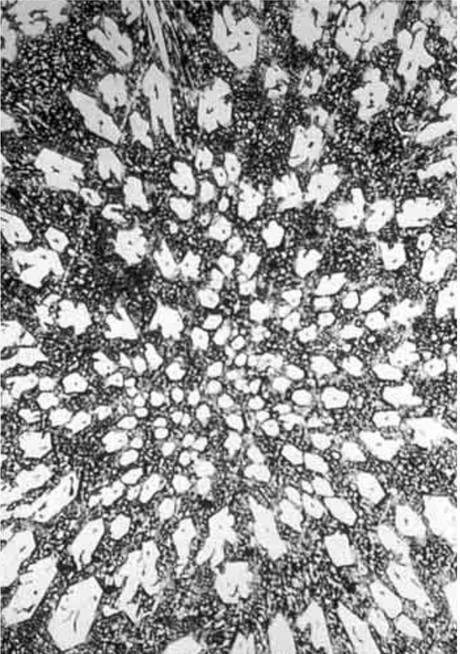
Microstructure hard-facing weld metal: OK 84.78, chrome carbide.
