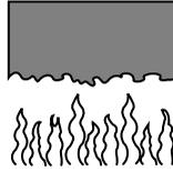
When metals are exposed to high temperatures for long periods, they generally lose their durability. High-temperature service often results in thermal fatigue cracking. For instance, thermal shock brought about by cyclic thermal stresses will occur in tools and dies designed for forging and hot working operations.
