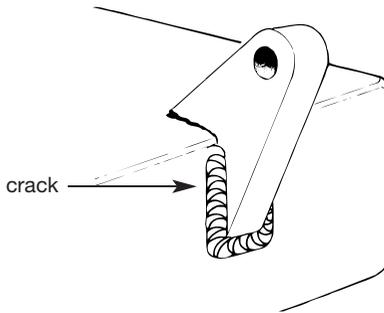
Repair of broken cast-steel support with OK 68.82.
