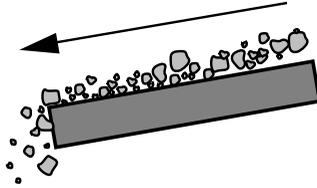
This type of wear is caused by sharp particles sliding or flowing across a metal surface at varying speeds and pressure, thereby grinding away material like small cutting tools. The harder the particle and the more sharp its shape, the more severe the abrasion.
