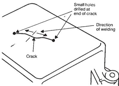
Procedure for repairing a crack
