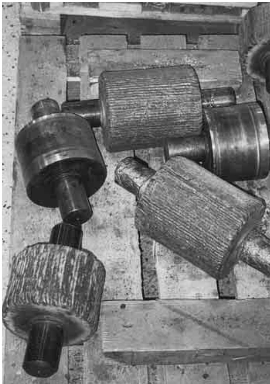
Hardsurfacing of support rollers OK 84.52 and OK 93.06.
