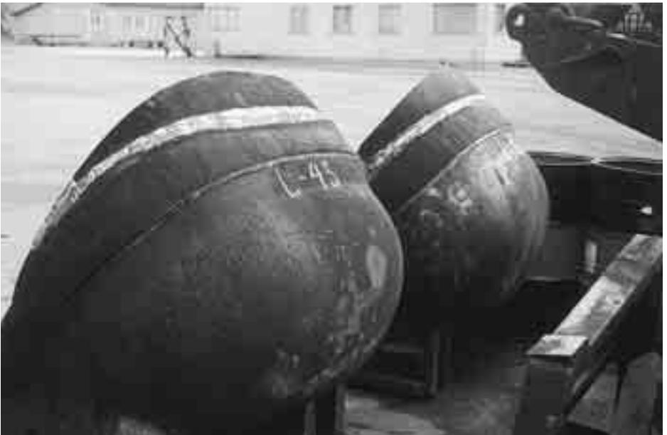
Dredger bucket. Joining new bucket lips using OK 68.82.
