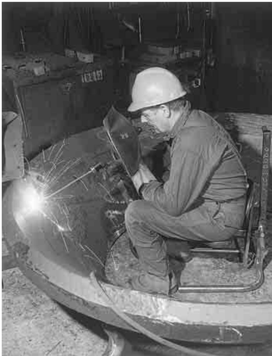
Repairing of 14% Mn steel crusher using OK 86.08.
